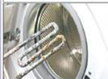
Heating Coils are getting Scales & the Heating time increased
