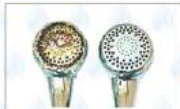
Showers are blocked due to Scales
