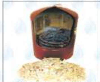
In Geysers the tubes are getting scales and the efficiency of the geyser decreased
